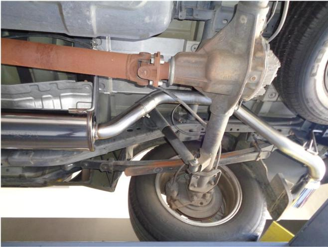
**Step 4.** Next loosely attach the Tail Pipe Assembly to the Muffler Assembly using the supplied clamp. Engage the welded hanger to the rubber insulator.
