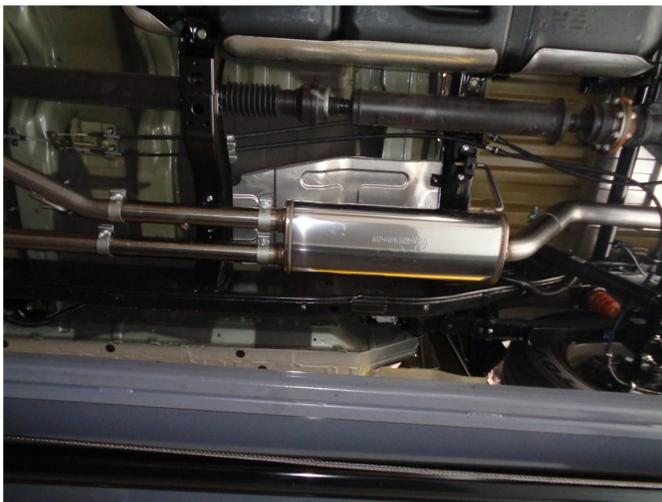
**Step 3.** Loosely attach the Muffler Assembly using the supplied clamps. Engage all welded hangers to the rubber insulators.
