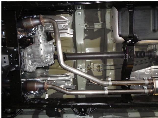
**Step 2.** Begin installation by loosely attaching the Inlet Pipe Assembly to the catalytic converter flange using the OEM hardware. Engage the welded hanger to the rubber insulator.
